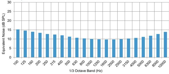
Figure 2: Typical Equivalent Noise under nominal conditions (Table 1)
