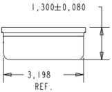
Notes: Metal can may be flush with, but not extend past, edge of microphone base on four sides.
